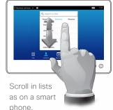
Tap the upper left corner to activate /deactivate the Do not disturb feature, to activate/ deactivate the Standby feature, and to access the Settings.
